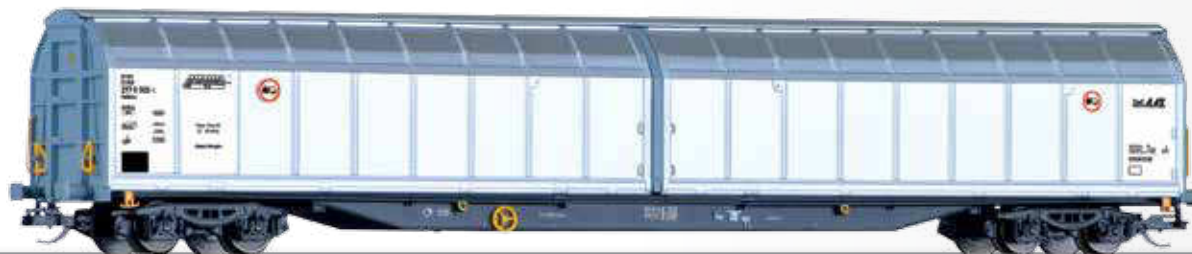
Schiebewandwagen Habbins der PKP Sliding cover box car Habbins of the PKP
