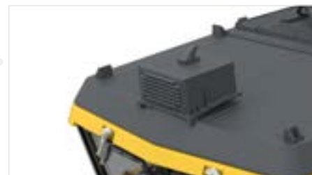
Separately attached signal horn box
