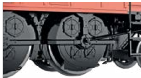
Prototypical representation of the "Buchli" drive
