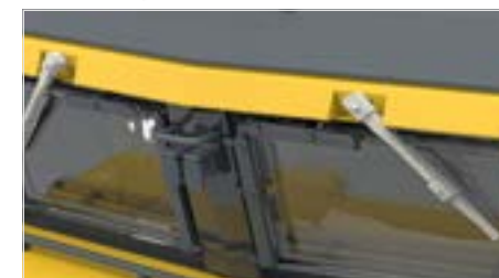
Plug-in windshield wipers and sockets
