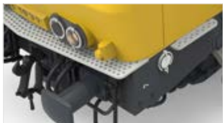
Running boards made from perforated metal
