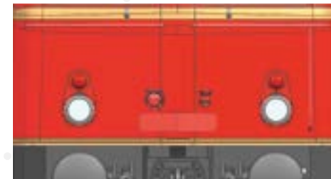
Separately attached sockets and running number
