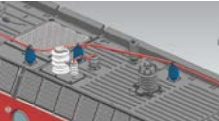
New main switch and primary voltage converter
