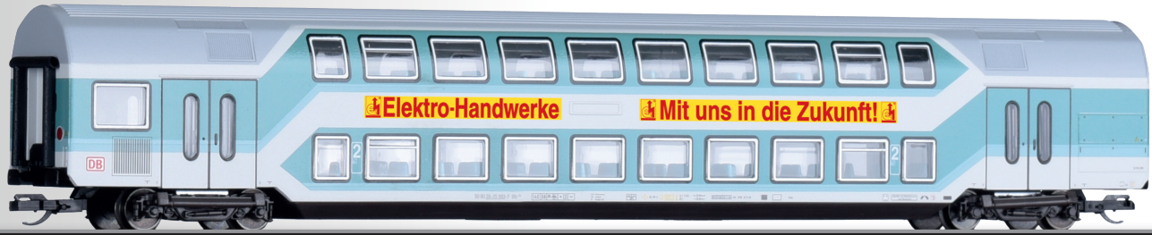
Doppelstockwagen 2. Klasse DBz 751 der DB AG 2nd class double-deck coach DBz 751 of the DB AG
